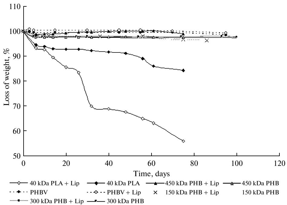
Fig. 1. Incubation of PHB, PLA and PHBV films in the absence and in the presence (+Lip) of lipase in Tris buffer, pH 7.7, at 37°C.
