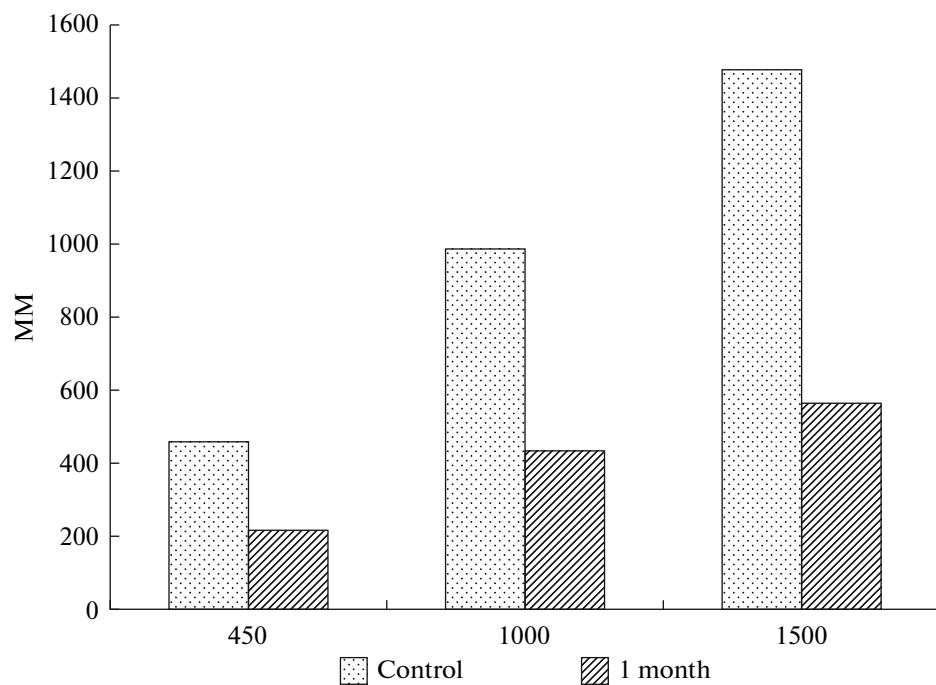
**Fig. 5.** Changes in molecular weight of PHB (450, 1000, and 1500 kDa) 1 month after their implantation to rats.
